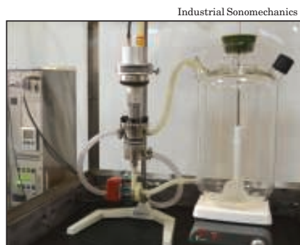
FIGURE 2. The BSP-1200 ultrasonic processor from Industrial Sonomechanics is designed for batch and flow-through processes and pilot-scale production. The processor outputs up to 1,200 W of acoustic power and operates at 20kHz
