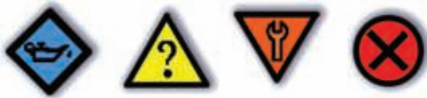
FIGURE 1. The NE 107 recommendation suggests standardized and easily understandable color and symbol conventions for status displays
